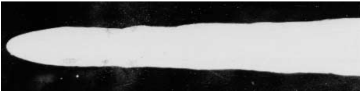
Fig. 7.17. Photographs from an experiment in which viscoplastic fluid (a mixture of water and joint compound) was extruded onto a sloping plane (inclined by roughly 30 degrees). Shown is the final shape after the extrusion was terminated and the fluid allowed to come to rest on the plane
