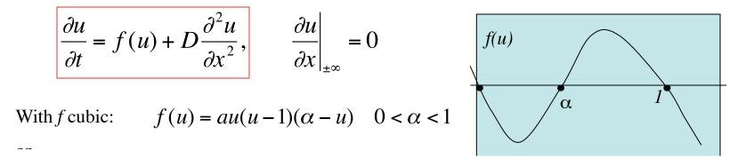
U is the shape of the wave, z is the position along the wave front
