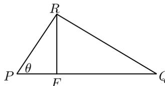
By the definition of the sine function, we have  $|RF|/|PR| = \sin \theta$ , so  $|RF| = |PR| \sin \theta$ . Now use the “one-half of base times height” formula to conclude that  $\triangle PQR$  has area  $(1/2)|PQ||PR| \sin \theta$ .
