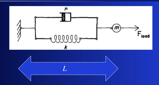
Elastic spring in parallel with a resistance ("dashpot")
