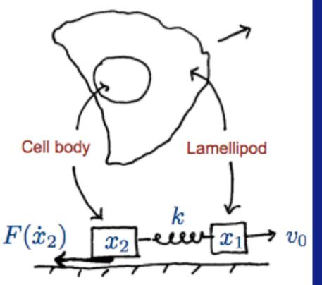
$$egin{array}{lll} d = x_1 - x_2 - L_0 & & \epsilon \dot{v} = kd - \xi_i v \ & & & & & & \\ v = \dot{x}_2 & & & & \dot{d} = v_0 - v \end{array}$$
