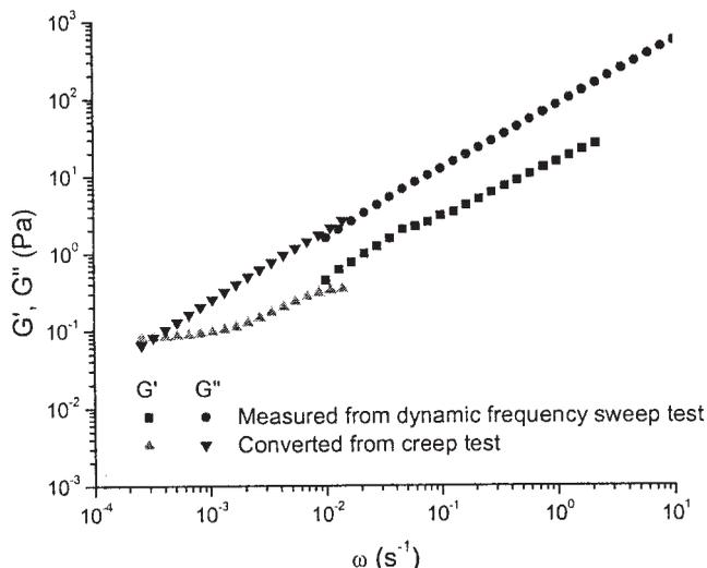
**Figure 6** Combined dynamic modulus of LC-5000 at 295°C.
