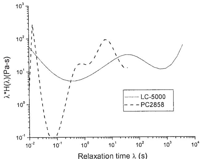
**Figure 7** Weighted relaxation spectrum of LC-5000 and PC2858 at 295°C.
