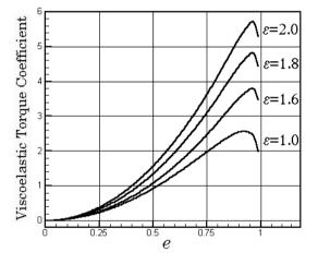
Fig. 6. Viscoelastic torque coefficient  $\mathcal{G}_{\mathcal{V}}^{(\varepsilon)}$  vs. eccentricity *e* for different values of  $\varepsilon$ .
