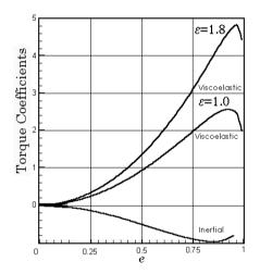
Fig. 8. Comparison of the inertial torque coefficient to the viscoelastic torque coefficient, for different values of  $\varepsilon$ . The viscoelastic torque coefficient is almost five times larger than the inertial one for e around 1 (slender ellipsoids) and  $\varepsilon = 1.8$ .
