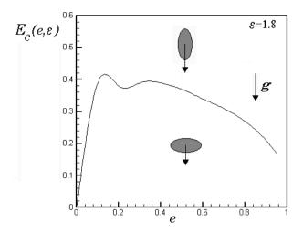
Fig. 5. Critical elasticity number  $E_c$  versus eccentricity e, for  $\varepsilon = 1.8$ . If  $E > E_c$  the ellipsoid falls with its major axis a parallel to  $\mathbf{g}$ , while if  $E < E_c$ , the fall with a parallel to  $\mathbf{g}$  is stable.
