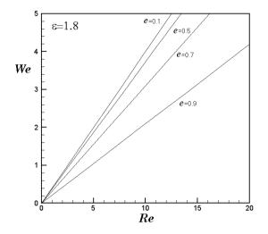
Fig. 9. Critical ratios of inertial versus viscoelastic torques for varying eccentricities e.
