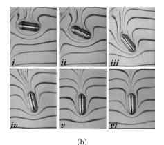
Fig. 1. Orientation of cylinders with round ends in a Newtonian liquid at nonzero Reynolds number (a), and in a purely viscoelastic liquid at vanishingly small Reynolds number (b).<sup>17</sup> In the Newtonian case (a) the initial configuration is with the major axis parallel to the gravity (unstable) and the terminal configuration is with the major axis perpendicular to the gravity (stable). In the purely viscoelastic case (b) the situation is reversed.
