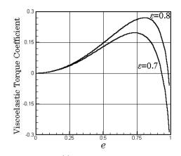
Fig. 7. Viscoelastic torque coefficient  $\mathcal{G}_{\mathcal{V}}^{(\varepsilon)}$  versus e, for  $\varepsilon = 0.7, 0.8$ . The torque coefficient changes sign for e at approximately 0.9. Note also that the curves achieve their peaks at decreasing values of e as  $\varepsilon$  decreases.
