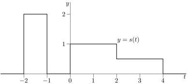
We can write this signal as a sum of rectangular pulses. As we saw in the last example,  $r_{HWC}(t) = H \operatorname{rect}(\frac{t-C}{W})$  is a single rectangular signal with height H, centre C and width W. So
