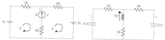
Questions A25 and A26 concern the circuits above. In the left diagram, I is the current through the current source and E is the voltage across it, to be determined.
