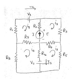
A20: Consider the resistor network above. Using the loop current method you have learned in the lectures and labs, write the equation for voltages around loop 1. Your equation should have the resistances and sources as parameters.
