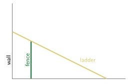
Suppose a 2-metre high fence stands 1 metre away from a high wall. What is the shortest ladder that will reach over the fence to the wall?
