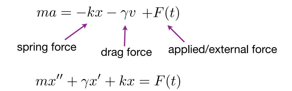
Forced vibrations - nonhomogeneous linear equation with constant coefficients.
