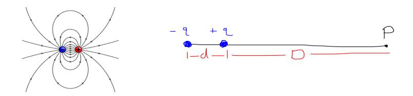
Approximate the *E*-field at distance  $D \gg d$  from a dipole (figure):
