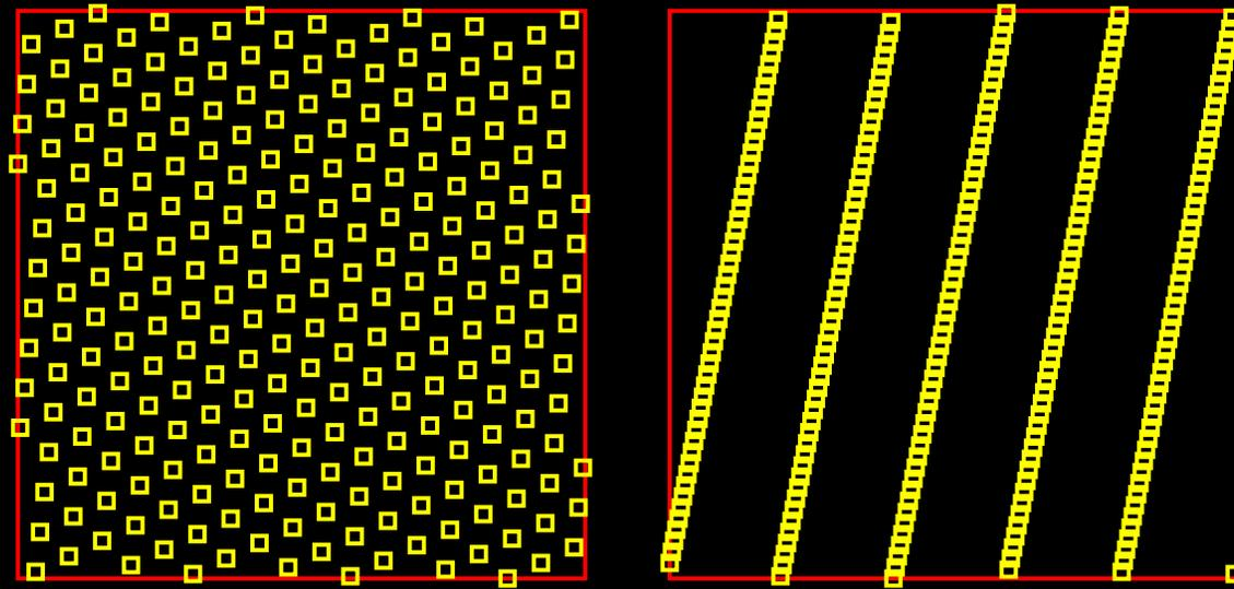
**A generator is measured by the maximum distance between systems of ‘planes’ containing the plots, or equivalently by the length of shortest vectors in the dual lattice. Shorter dual vectors means greater ‘planar’ spacing, so we want the shortest vector not to be too short.**
