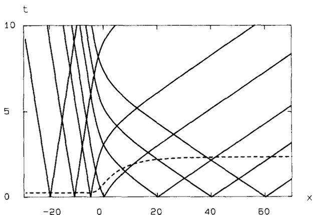
FIG. 5. Characteristic curves, defined by  $dx/dt = \pm c(x)$ , emanating from the  $x$  axis, are plotted for  $\nu = 1.4$ .
