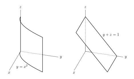
*E* is constructed by using the plane y + z = 1 to chop the top off of the parabolic cylinder  $y = x^2$ . Here is a sketch.
