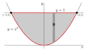
By definition, the centre of mass is  $(\bar{x}, \bar{y})$ , with  $\bar{x}$  and  $\bar{y}$  being the weighted averages of the x and y-coordinates, respectively, over D. That is,
