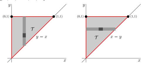
First, we'll set up the integral using vertical strips. Looking at the figure on the left above, we see that, on T,
