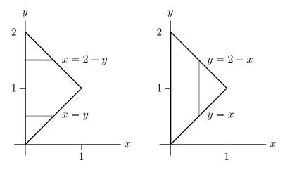
To reverse the order of integration, we decompose the domain using vertical strips as in the figure on the right above. As
