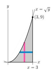
The inside integral,  $\int_{\sqrt{y}}^{3} \sin(\pi x^3) dx$ , in the given integral looks really nasty. So let's try exchanging the order of integration. The given integral was formed by decomposing the domain of integration *D* into horizontal strips, like the blue strip in the figure above. To exchange the order of integration we instead decompose the domain of integration *D* into vertical strips, like the pink strip in the figure above. To do so, we observe that, on *D*,
