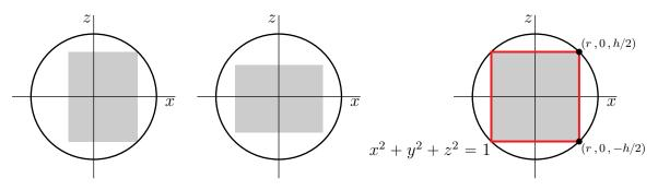
So we are to maximize the volume,  $f(r,h) = \pi r^2 h$ , of the cylinder subject to the constraint  $g(r,h) = r^2 + \frac{h^2}{4} - 1 = 0$ . According to the method of Lagrange multipliers,
