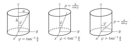
For each fixed  $\varphi$ ,  $\theta$  runs from 0 to  $2\pi$  and  $\rho$  runs from 0 to either  $\frac{h}{\cos \varphi}$  (at the top of the
