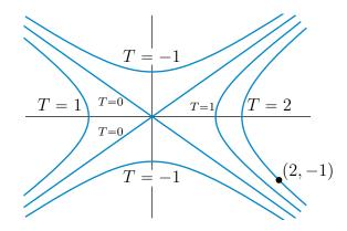
Note that the temperature gradient is  $\nabla T(x, y) = \langle 2x, -4y \rangle$ . In particular, the temperature gradient at (2, -1) is  $\nabla T(2, -1) = \langle 4, 4 \rangle$ .
