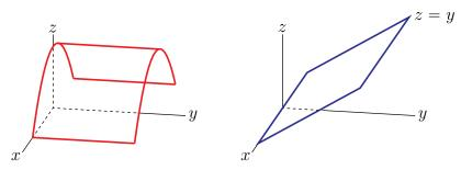
(b) The figure on the right above is a sketch of the plane y = z. It intersects the surface  $z = 1 - x^2$  in the solid blue sloped parabolic curve in the figure below.
