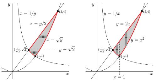
(b) To reverse the order of integration we use vertical strips as in the figure on the right above. Looking at that figure, we see that, on *R*,
