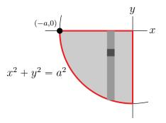
• Finally, the inside integral says that, for each (x, y) in the quarter disk, z runs from 0 to  $\sqrt{a^2 - x^2 - y^2}$ . We can also rewrite  $z = \sqrt{a^2 - x^2 - y^2}$  in the more familiar form  $x^2 + y^2 + z^2 = a^2$ ,  $z \ge 0$ .
