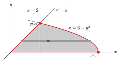
The bottom slice has y = 0 and the top slice has y = 2. On the slice at height y, x runs from y to  $6 - y^2$ . So
