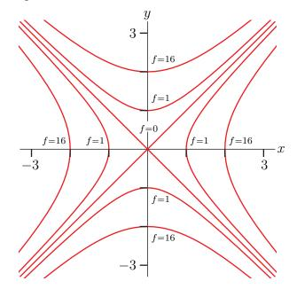
(b) As  $f_x(x,y) = -4x(y^2 - x^2)$  and  $f_y(x,y) = 4y(y^2 - x^2)$ , we have  $f_x(0,0) = f_y(0,0) = 0$  so that (0,0) is a critical point. Note that
