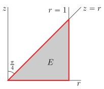
Recall that the spherical coordinate  $\varphi$  is the angle between the *z*-axis and the radius vector. So, in spherical coordinates z = r (which makes an angle  $\frac{\pi}{4}$  with the *z* axis)
