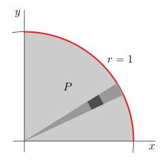
By symmetry under reflection in the line y = x, we have  $\bar{y} = \bar{x}$ . So we just have to determine
