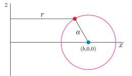
$(r-b)^2 + z^2 = a^2$ . (Recall that the cylindrical coordinate *r* of a point is its distance from the *z*-axis.) On this torus,
