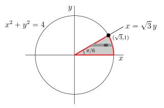
(b) In polar coordinates, the circle  $x^2 + y^2 = 4$  is r = 2 and the line  $x = \sqrt{3}y$ , i.e.  $\frac{y}{x} = \frac{1}{\sqrt{3}}$ , is  $\tan \theta = \frac{1}{\sqrt{3}}$  or  $\theta = \frac{\pi}{6}$ . As  $dx dy = r dr d\theta$ , the domain of integration is
