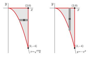
(b) The inside integral,  $\int_{\sqrt{-y}}^{2} \cos(x^3) dx$  looks nasty. So let's reverse the order of integration and use vertical, rather than horizontal, slices. From the figure on the right above, on the domain of integration,
