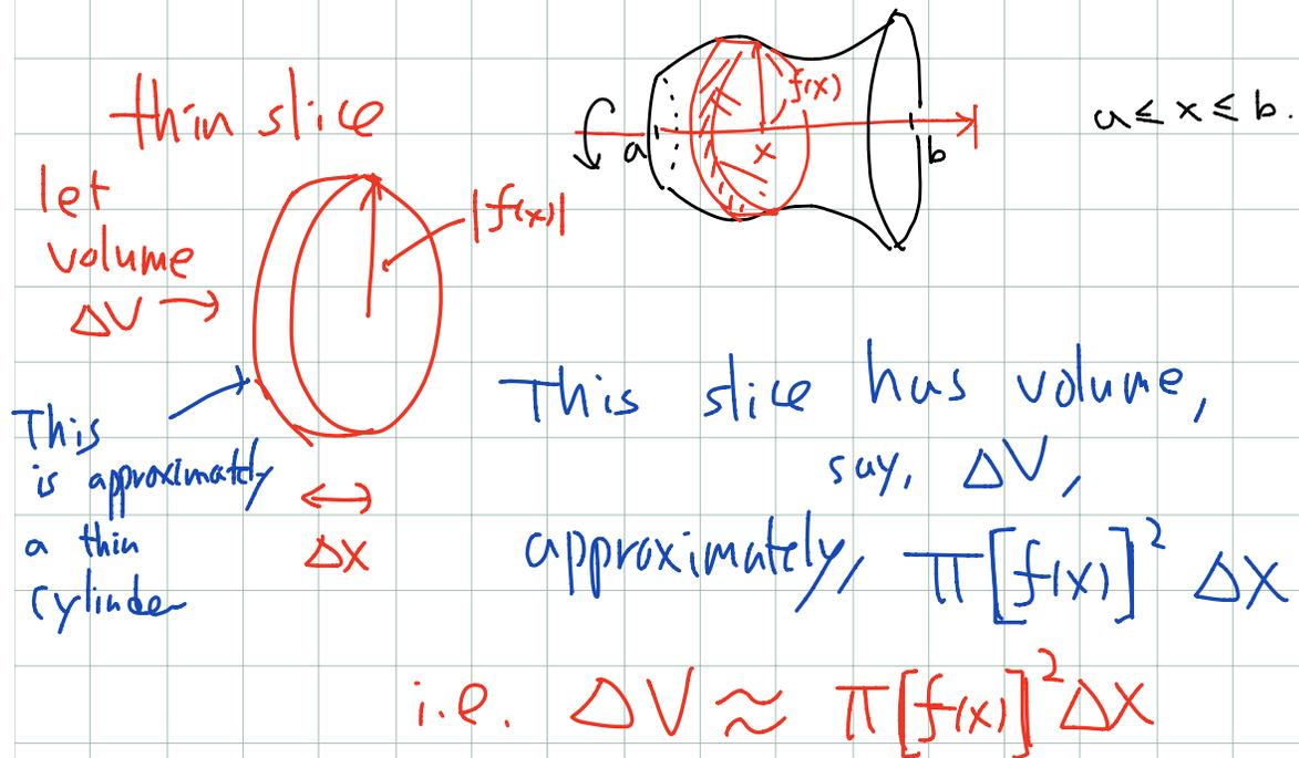
The diagram shows a solid of revolution on the right, formed by rotating a curve around the x-axis from  $x=a$  to  $x=b$ . A thin slice is highlighted in red, with its radius labeled  $|f(x)|$  and its thickness  $\Delta x$ . To the left, a separate drawing of a thin cylinder is shown, with its radius also labeled  $|f(x)|$  and its thickness  $\Delta x$ . The text explains that the volume of this slice is approximately  $\pi [f(x)]^2 \Delta x$ .
