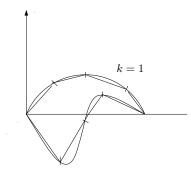
Richardson Extrapolation:  $\lambda_k = \lambda^e + c_2 h^2 + c_4 h^4 + \dots$
