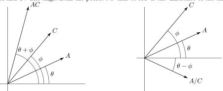
Complex numbers are also called "phasors" by some electrical engineers. They call the diagrams resulting from the geometric evaluation, as above, of algebraic expressions involving complex numbers "phasor diagrams". For example, suppose that an AC signal of frequency  $\omega$  is applied to the left hand end of the parallel circuit
